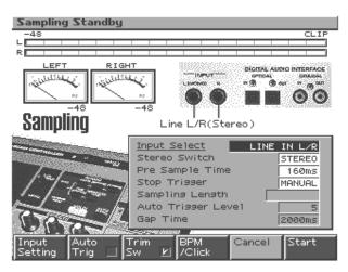
3. Make the settings for things such as the input source of the sound to be sampled, and triggering.
